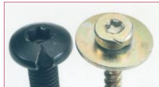
Typical forging cracks.
